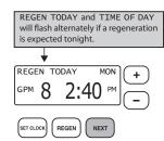
For Immediate Regeneration: Press and hold **REGEN** until valve motor starts (typically 3 seconds).
